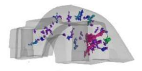
In every day operations simplicity is the key. To ensure an efficient workflow the image acquisition is a native feature of the **Xplus Handle**. The reconstruction and analysis takes part in the renown VGStudio, which is the industry standard. Typical applications are actual-nominal comparison, porosity analysis, measurement and CAD comparison. Combined with a robot even complex 3D ADR inline inspections become reality.
