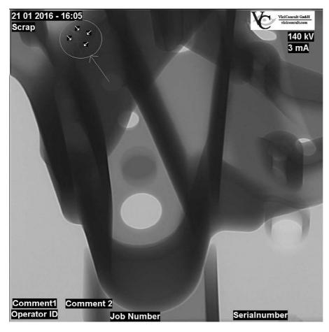
The VisiConsult overlay toolbox is a standard module that offers a broad variety of choices. This leads to a huge increase in efficiency compared to placing lead numbers on every shot.
