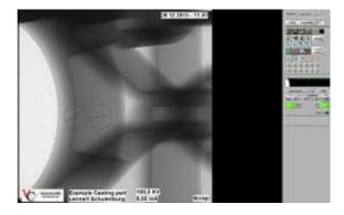
The Live Filters are a powerful toolbox that allow to spread the grey values to look into areas with different wall thickness for a convenient inspection. At the same time defects will be highlighted by a contrast filter for an enhanced optical inspection. The effect of all these fine-tuned algorithms is activated by a single click.
