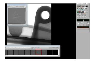
If there are still doubts the reference defect can be directly projected into the current X-ray image for best comparison. The operator can choose the defect type and size from an image browser. All official defect types like shrinkages, porosities, cracks and many more are covered through this module.
