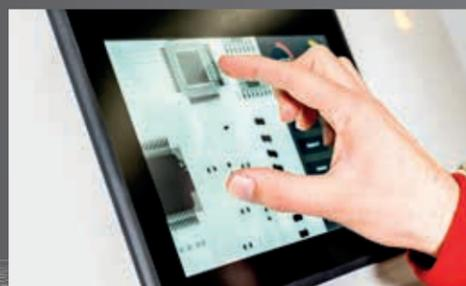
The InSpect cabinet is equipped with a high resolution touch panel for fast and intuitive operation. All main functions of the system like energy, current and exposure time can be set within seconds. Commonly used parameters can be easily stored.
