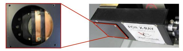
To collimate the X-ray beam VisiConsult developed a set of diaphragms that can be used on the tube or detector side. This prevents blooming, protects unshielded areas of the specimen or detector and can reduce the range of grey values. There are various customizable choices available: 2 axes rectangular, iris shape and many more.
